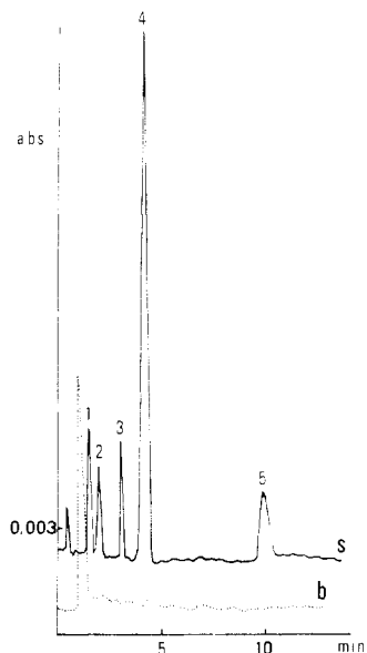
Figure 1. HPLC chromatogram of lettuce blank (b, dotted line) and of a standard mixture of pesticides (s). Peaks: (1) cymoxanil (1.0 ppm); (2) BMC (1.0 ppm); (3) benomyl (1.0 ppm); (4) thiram (3.0 ppm); (5) vinclozolin (1.5 ppm). Chromatographic conditions: column RP-18, mobile phase H 2 O-CH 3 CN, 50:50, plus 0.6% NH 3 ; flow rate 1.5 mL/min; sample size 50 μL; UV detector at 220 nm; 0.032 AUFS; temperature 30 °C.
